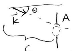
$$I(\omega, T) = \frac{c}{2} A u(\omega, T) \underbrace{\frac{1}{4\pi} \int d\Omega \cos\theta}_{2\pi} = \frac{c}{4} A u(\omega, T)$$
