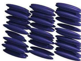
Figure 6.5: Cartoon of a Liquid Crystal. Liquid crystals have some of the properties of a solid and some of the properties of a liquid. In this picture of a smectic-C liquid crystal the system is crystalline in the vertical direction (forming discrete layers) but remains liquid (random positions) within each plane. Like a crystal, in this case, the individual molecules all have the same orientation.
