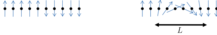
Figure 20.4: Domain Wall Structure. Left: An infinitely sharp domain wall. This would be realized if the anisotropy energy ( \kappa ) is extremely large so the spins must point either up or down (i.e., this is a true Ising system). Right: A Bloch/Néel wall (actually this depicts a Néel wall) where the spin flips continuously from up to down over a length scale L . The anisotropy energy here is smaller so that the spin can point at intermediate angle for only a small energy penalty. By twisting slowly the domain wall will pay less spin-stiffness energy.
