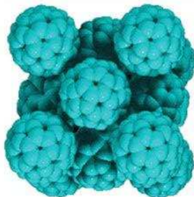
Figure 6.2: A Molecular Crystal. Here, 60 atoms of carbon bind together to form a large molecule known as a buckyball 2 , then the buckyballs can stick together to form a molecular crystal.
