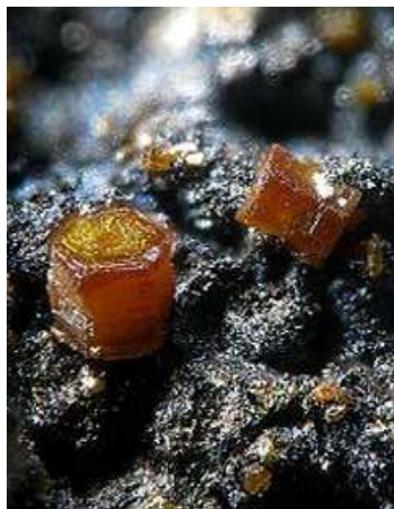
Figure 15.8: Orange crystals of CdS. This particular crystal is the naturally occurring mineral called “Greenockite” which is CdS with trace amounts of impurity which can change its color somewhat.
