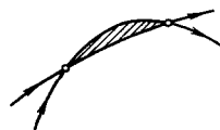
FIG. 39. Electrons moving on neighboring paths interfere and this leads to oscillations in transport characteristics. The period in the magnetic field is determined by the shaded region. Points represent the region of magnetic breakthrough.
