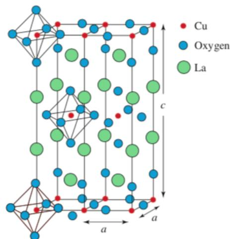
**Fig. 1** Crystal structure of  $\text{La}_2\text{CuO}_4$ , showing body-centered tetragonal conventional cell
